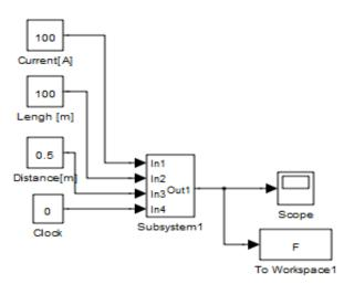
Fig.1. Simulink model for single-phase short circuit
