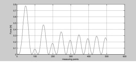
Fig.2. Force diagram for single-phase short circuit
