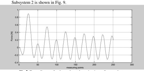
Fig.5. Force diagram for three-phase short circuit, median conductor
