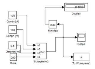
Fig.4. Simulink model for three-phase short circuit, median conductor
