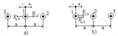
Fig.3. Disposition of conductors in the same plane: a) Forces exerted on the median conductors b) Forces exerted on the side conductor
